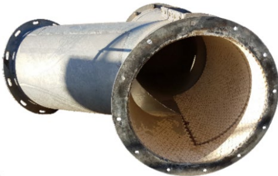
Wear pads installed in grain transfer pipes
